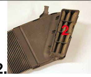
Remove the filter from the inlet pipe. (2).
