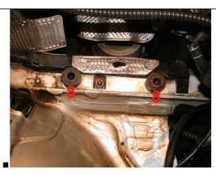
Replace the rubber bushings if needed (8).
