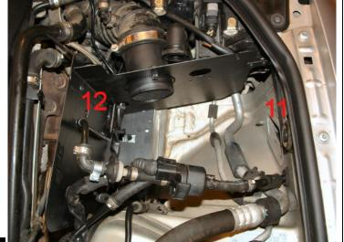
Attach shield B to shield A, use the M5 screws and nuts, put the pipe and harness threw the hole (12).
