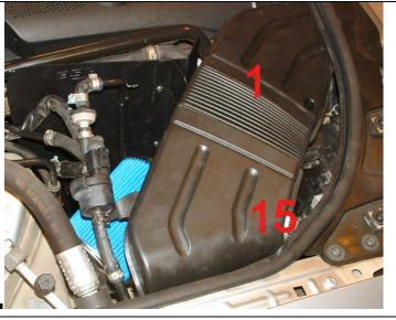
Assemble the inlet pipe (1).
