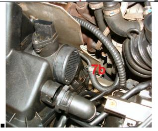
Remove the lower hose clamp (7b) for the EVAP-pipe And loosen the hose.
